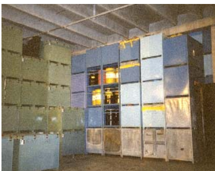
Figure 1.a. LLRW storage containers Source: Ontario Power Generation
