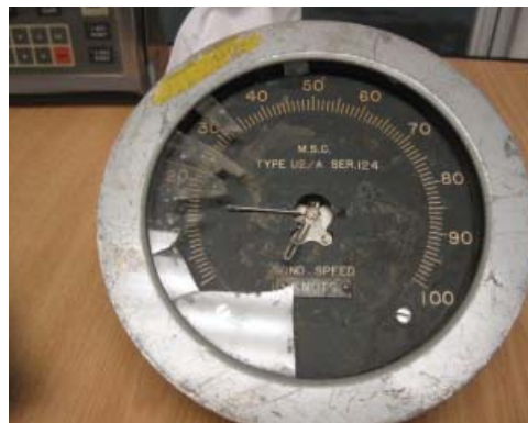
The writing on this broken aircraft dial (left) and the tips of the toggle switches (bottom), used to glow in the dark with radium luminous paint.
