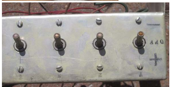
The writing on this broken aircraft dial (left) and the tips of the toggle switches (bottom), used to glow in the dark with radium luminous paint.
