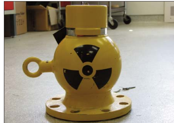
Image #7: Industrial fixed gauge
