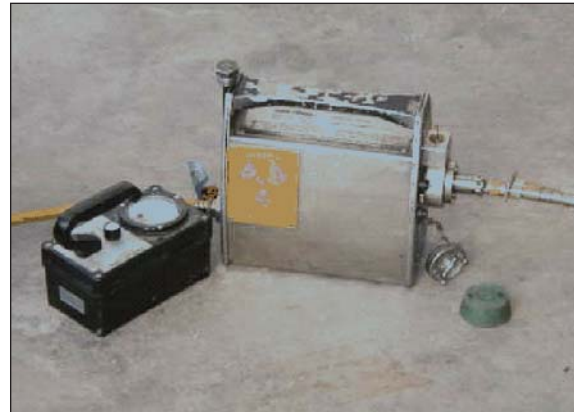
Image #5: Industrial radiography camera which contains the radioactive sealed source
